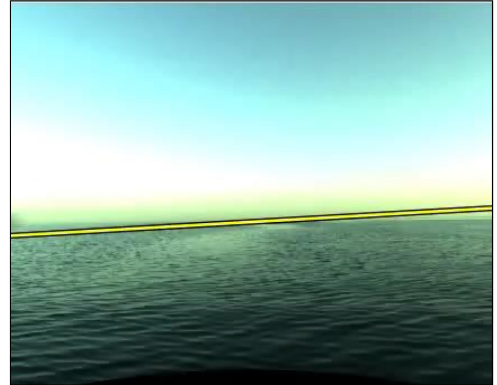
Camera tilt estimated from IMU, horizon projected into image
